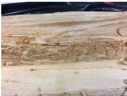
Figure 3. Carpenterworm frass/tunneling damage.
